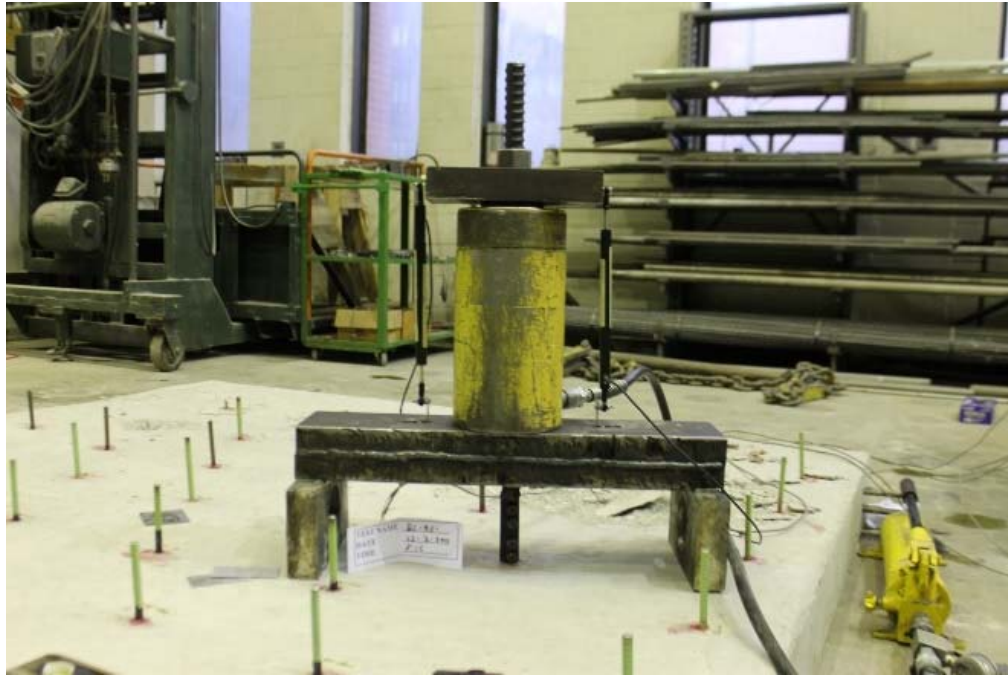
Figure B.49 Complete assembly and specimen prior to testing for BL-BE-1
