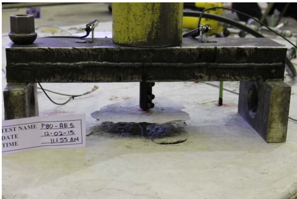
Figure B.47 Detailed view of the reinforcement at failure for P80-AE-5
