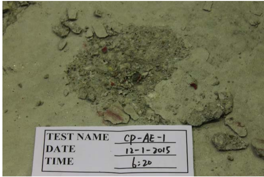
Figure 4.12 Representative failure mode for CP-AE of combined failure (concrete breakout and steel rupture)
