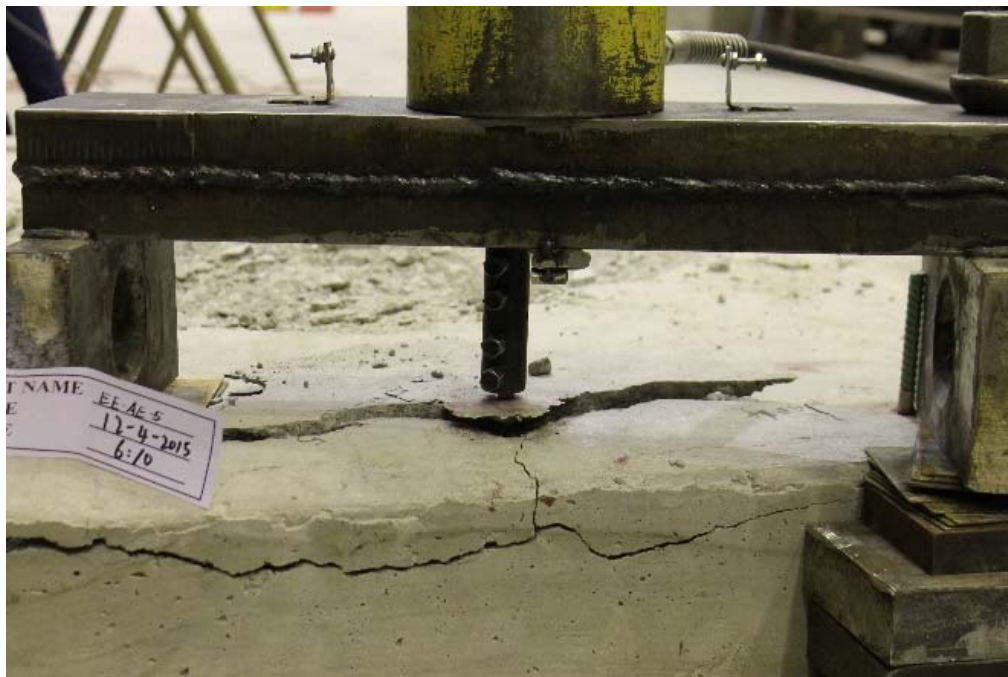
Figure B.62 Detailed view of the reinforcement at failure for EE-AE-5
