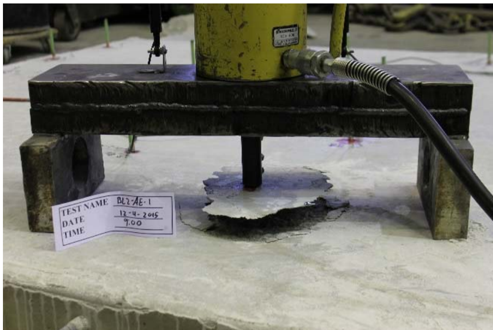
Figure B.2 Detailed view of the reinforcement at failure for BL-AE-1
