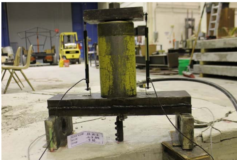
Figure B.58 Complete assembly and specimen prior to testing for EE-AE-3
