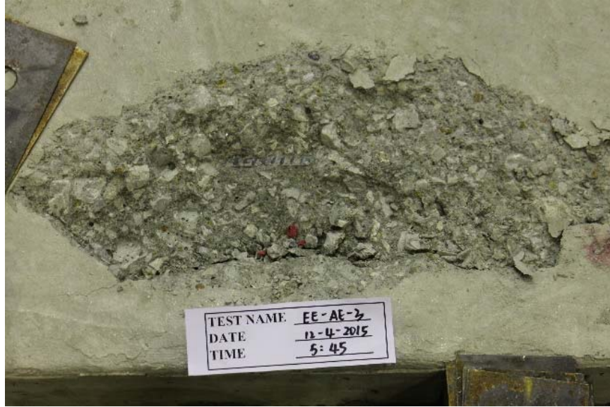
Figure 4.20 Representative failure mode for EE-AE of side concrete blowout
