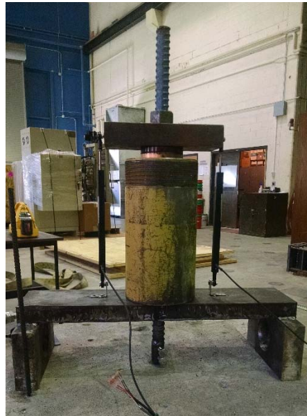
Figure 3.9 Test setup with yellow hydraulic jack, rebar coupler, Dywidag, and two LVDTs
