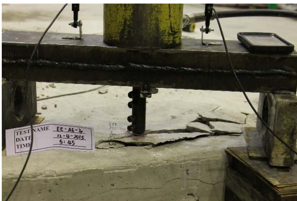
Figure B.59 Detailed view of the reinforcement at failure for EE-AE-3
